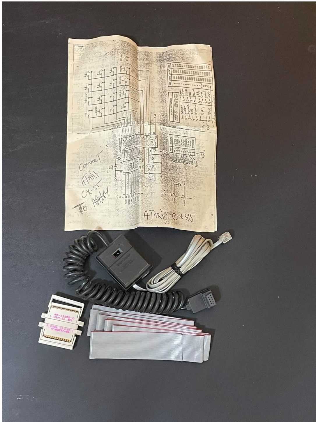
Fig 5. Kit as received. The annotated Atari CX-85 service schematic (top), the keypad itself with its coiled cable and plug, the modular/RJ cable, two Winchester IDC-to-edge sockets, and several lengths of grey ribbon cable.
